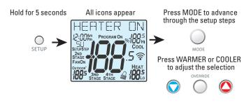
Technician Setup is for diagnostic and testing purposes and is intended for use by a qualified technician. See next page for more detailed instructions.
