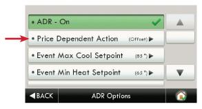
Selecting the 'Price Dependent Action' button allows the user to determine what action is taken when the price rises above the set threshold.
