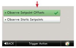
In the above example; if the price threshold is exceeded, the thermostat will invoke the 'Offset Setpoints' configured for an ADR event until the event is over.
