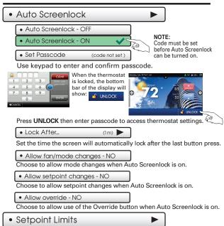
Limits how high or low heating and cooling may be adjusted.
