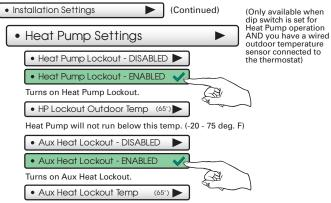
Aux Heat will not run above this temp. (0 - 75 deg. F) **GAS/EL** or **HP** dip switch must be set for **HP** and **GAS** or **ELEC** dip switch must be set for **ELEC**.
