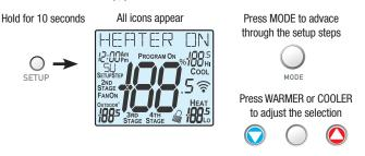
Technician Setup is for diagnostic and testing purposes and is intended for use by a qualified technician. See next page for more detailed instructions.
