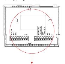
To remove the thermostat backplate from the wall: pry with screwdriver in either slot to remove back plate
