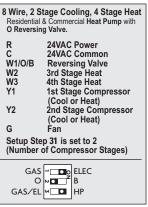
Note: When the unit goes into 4th stage heating, there is no 4th stage indicator, the display will still show 3rd stage.
