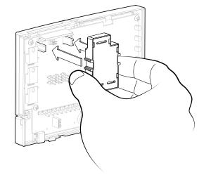
3. Carefully press the front housing with installed WiFi module back on to the backplate.
