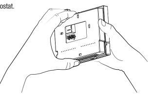
Install the Wi-Fi module as shown onto the printed circuit board.
