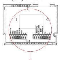
To remove the thermostat backplate from the wall: pry with screwdriver in either slot to remove back plate
